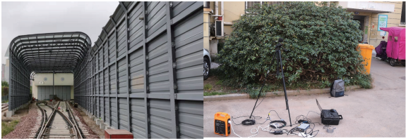
图 11 地铁出入线轨道、声屏障及现场噪声测试照片 Figure 11 Photos of metro access line tracks, sound barriers and in-situ noise measurement
