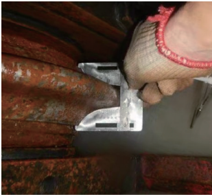
图 4 刀圈磨损量测量示意图 Figure 4 Illustration of cutter ring wear measurement
