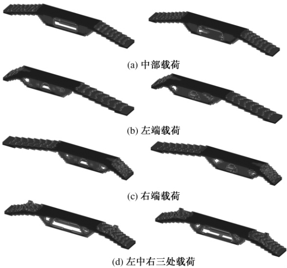
图 5 不同工况不同过滤函数简支梁拓扑优化结果 Fig. 5 Simply supported beam's topology optimization results with different loads and filters
