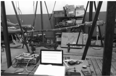
图 4 排气管的自由模态试验安装与测试 Fig. 4 Free modal experiments installation and test of exhaust pipe
