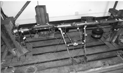
图 7 BBC 总成安装 Fig.7 The BBC assembly installed
