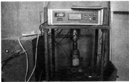
图2 应力吸收层层间剪切仪 Fig.2 Stress absorbing membrane interlayer shear apparatus
