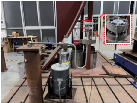
图 14 安装二重动力吸振器的小支管 Figure 14 Install the small branch tube of the double dynamic vibration absorber
