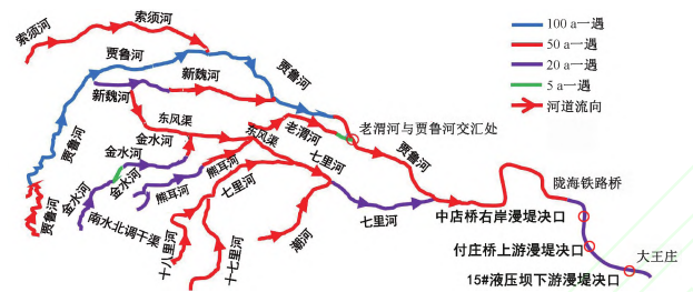
图 3 主城区河道现状排涝能力及贾鲁河下游决口位置示意图 Figure 3 Schematic diagram of current drainage capacity of river channels in the urban area and the location of the breach in the lower reaches of Jialu River
