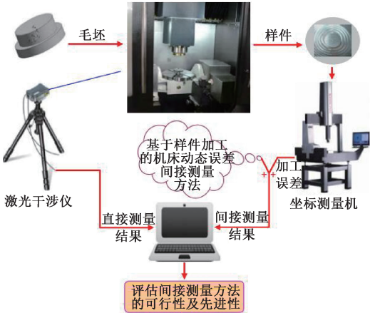
图 4 五轴数控机床动态误差间接测量方案 Figure 4 Five-axis CNC machine tool dynamic error indirect measurement scheme
