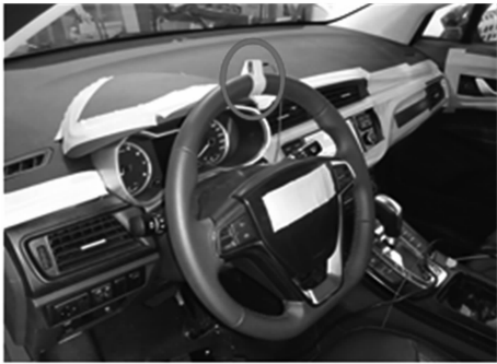
图 1 方向盘上振动传感器测点布置 Fig.1 Position of acceleration sensor on the steering wheel
